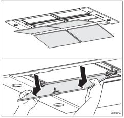
■ To remove a panel, hold it at the sides, as shown. Pull it downwards out of the front locking clip, unhook it at the back and remove it.
